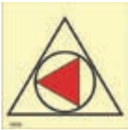
Remote control for fire pump(s)
