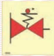
Remote controlled fuel/lubricating oil valves
