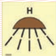
Space(s) protected by fire extinguishing system
