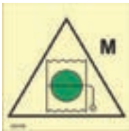
Remote control for fire damper(s)
