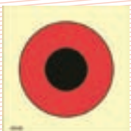
Push button/switch for general alarm
