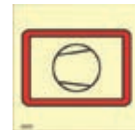
Air compressor for breathing devices
