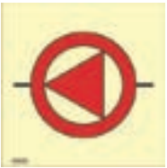
Emergency fire pump
