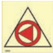
Remote control for emergency fire pump
