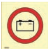
Emergency source of electrical power (battery)
