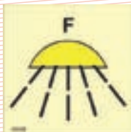
Space(s) protected by fire extinguishing system
