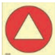
Space/group of spaces monitored by gas detector(s)
