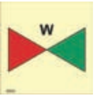
Fire main section valve
