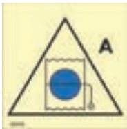
Remote control for fire damper(s)
